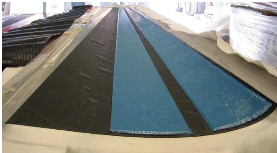
Figure 7-29: Top wing skin core sections with honeycomb encased in film-adhesive after placement and before addition of the top sandwich ply.
