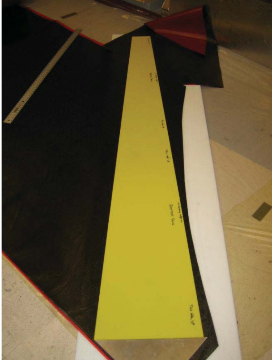
Figure 7-25: Wing skin laminate plies being cut to shape using a custom-made plastic template.
