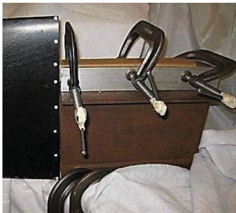
Figure 7-45: Detail of cantilever test fixture.
