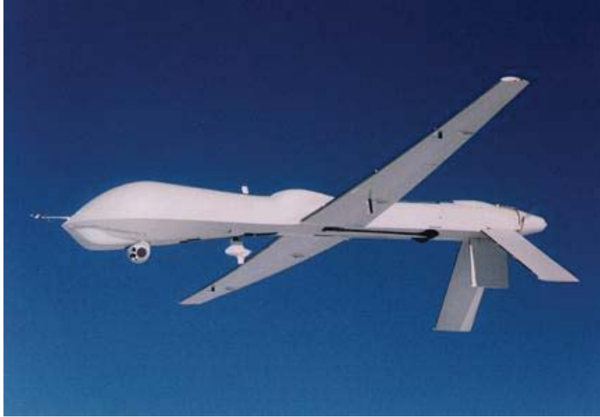
Figure 1-1: The all-composite Predator UAV by General Atomics.
