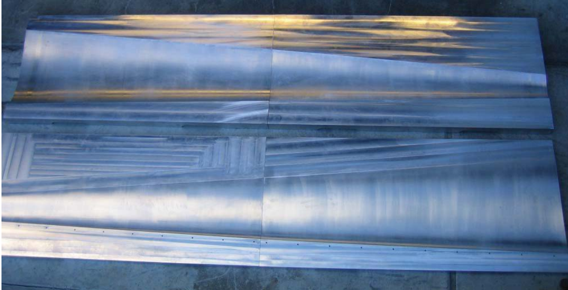
Figure 7-24: Machined aluminum molds for layup and cure of the composite wing skins.
