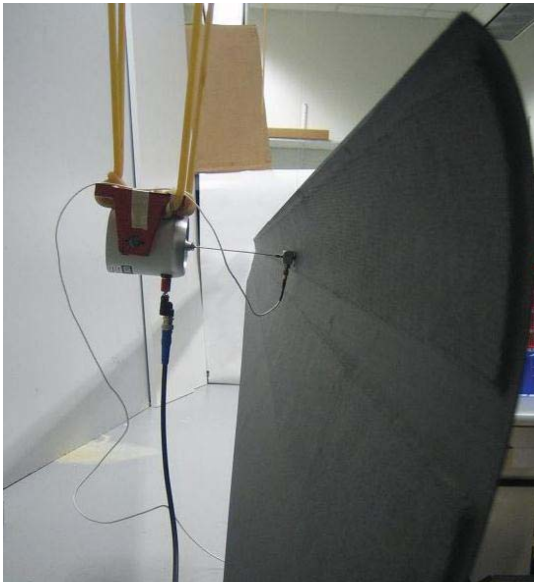
Figure 7-39: View of the electrodynamic shaker and force transducer attachment method, shown during component vibration testing of the top wing skin.
