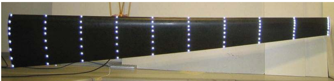
Figure 7-41: Top wing skin components in free-free scanning laser Doppler vibrometer modal testing configuration.
